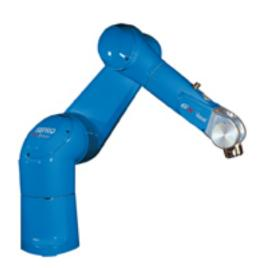
A Sepro 6X-90L 6-axis articulated-arm robot (left) and a Sepro Success 11 Cartesian beam robot with telescoping arm (above) can be seen in a live demonstration of insert loading and part removal at Plastec West 2019. The demo illustrates capabilities like insert pick-up and placement, part removal and accurate positioning for post-mold operations.
