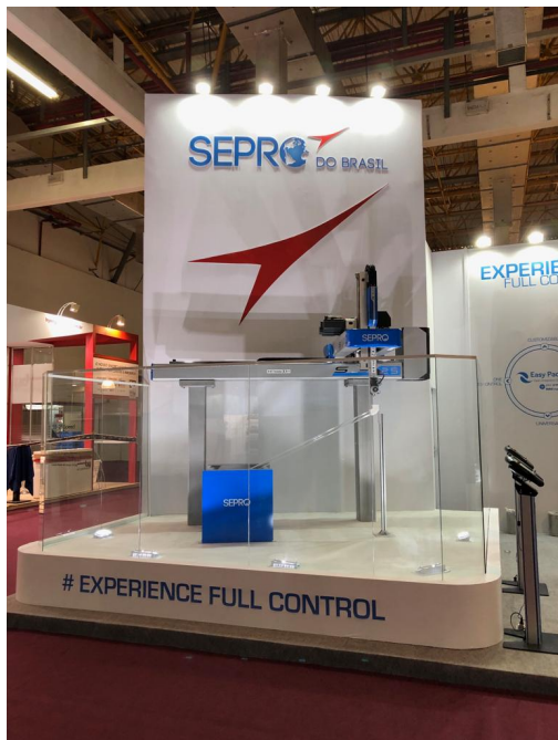
Being shown in Brasil for the first time, the 3-axis Sepro S5-25 Speed, was developed for molders seeking a high-speed robot to serve injection-molding machines from 120 to 450 tons.
