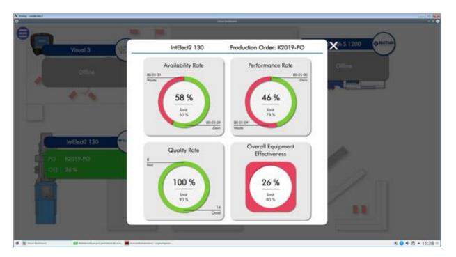
Sepro robot controls gather a lot of production data that can be used to calculate OEE and other metrics for presentation on the new Visual Dashboard.
