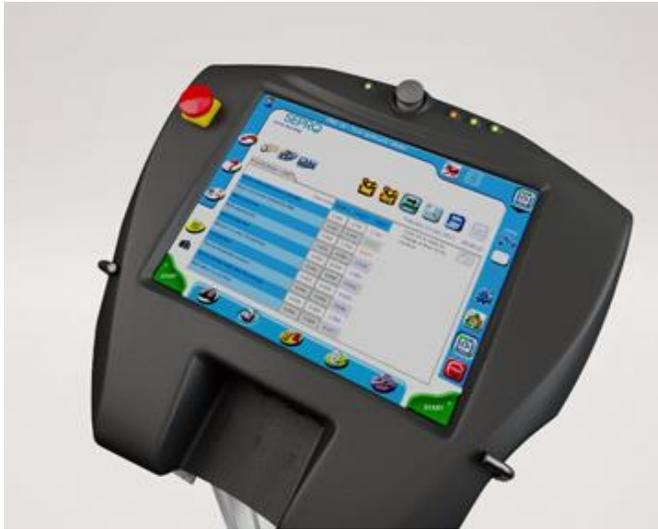
*OptiCycle, a plug-in for the Sepro Visual control, can envision the entire robot cycle, then break the program down into its component elements. Within each element, it offers programming instructions and best practices to guide the operator. Download a high-resolution image at: <http://tinyurl.com/Opticycle>*
