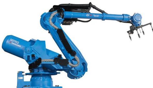
*The 6X-400 6-axis articulated-arm robot, the product of a recent manufacturing partnership with Yaskawa Motoman, has a 4m reach and can carry a maximum 120-kg payload. Download a high-resolution image at: <http://tinyurl.com/hbl8vap>*
