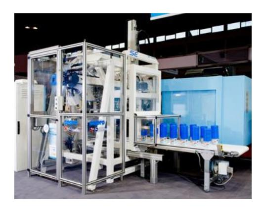
The Sepro IML demonstration cell on the Sumitomo Demag stand is molding 1.2-I pails with wrap-around labels in a 2-cavity tool on a 4.5-sec cycle.
