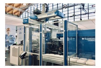
One of the two automation cells on the Sepro stand will feature a Sumitomo Demag molding machine equipped with an SDR Speed 7 robot. Made by Sepro especially for sale with Sumitomo Demag machines, this robot is capable of getting in and out of the mold space in under 1 sec. Download a high-resolution file: <u>https://tinyurl.com/SRO-Speed7</u>
